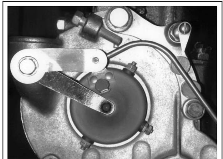
Figure 3—Timer Mounted on Engine Using Original Ford
