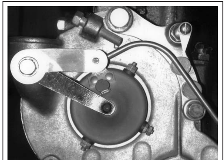
Figure 3—Timer Mounted on Engine Using Original Ford Adjustment Gauge Photo Courtesy of Steve Coniff
